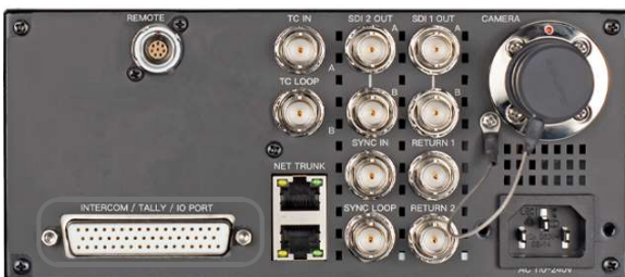
Intercom/Tally/GPIO DB50 interface
